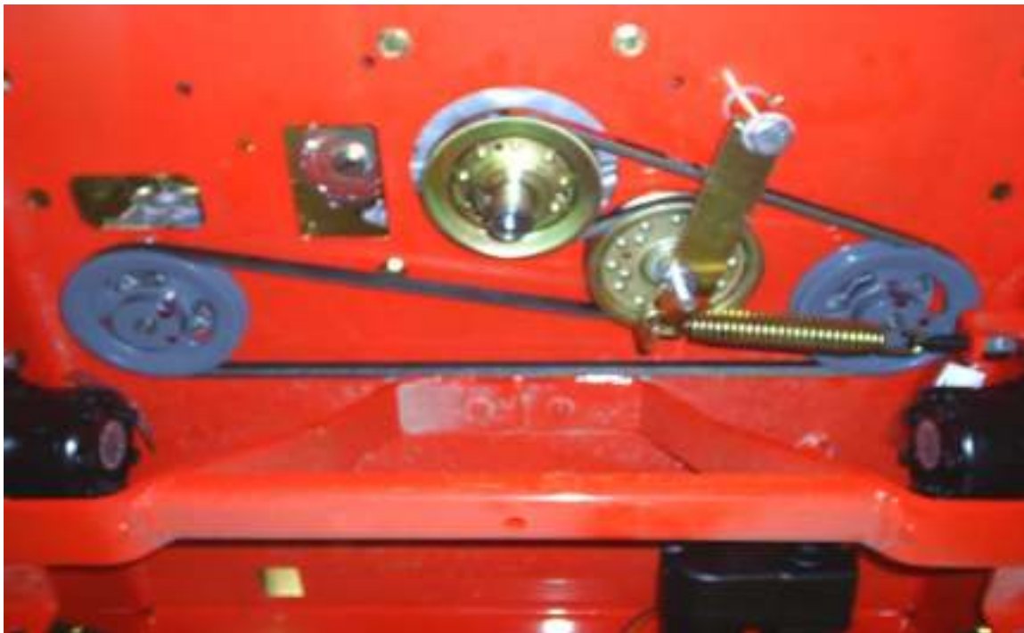
Shown above is a typical pump belt layout for most models.
