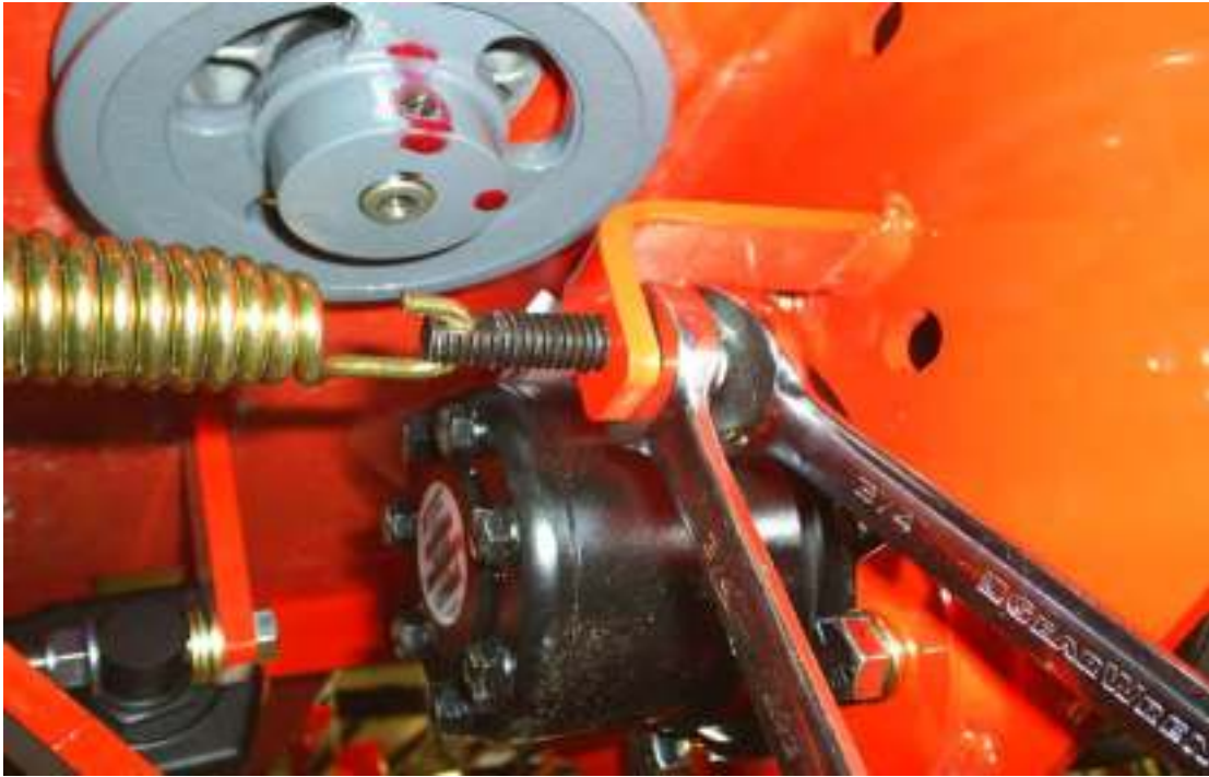
Shown above is a typical pump belt tensioner for ZT, Pup, Lightning, and Outlaw models.
