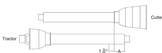
Do not use tractor if proper driveline engagement cannot be obtained through these methods. Connect driveline to tractor PTO shaft, making sure the spring-activated locking pin slides freely and locks driveline to PTO shaft.
