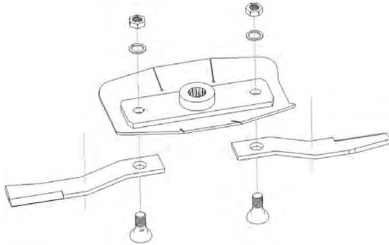
If blade bolt is seized in stump jumper's crossbar and extreme force will be needed to remove it, support crossbar from below to prevent gearbox damage.
