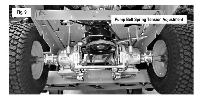
The tension should be adjusted so that there is between 60 to 65 lbs. of tension on the belt and <u>recheck belt tension after half an hour</u>. This can be checked with a belt tension gauge (Part Number 041-9999-00) as shown in Fig. 10.
