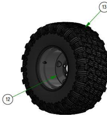
022-4091-00 REAR WHEEL ASSEMBLY 54" DECK
