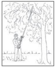
The shaft should always be held at an angle of  $60^{\circ}$  or less! The most convenient working position is a tool angle of  $60^{\circ}$ , but any lesser angle may be used to suit the situation concerned.
