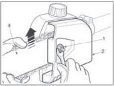
Check the chain tension. The tension is correct when the drive links do not slip out of the chain guides if you hold the chain in the middle of the bar.
