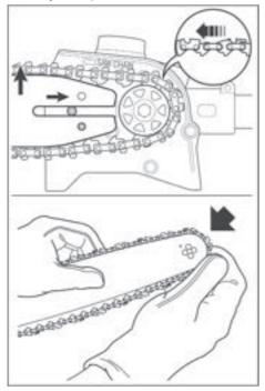
Check that the chain tension adjuster pin (5) is fitted properly in the hole on the bar; if it isn't, turn the chain tension adjuster screw (6) using a screwdriver until the pin is completely inserted.
