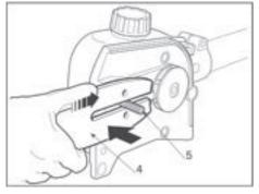
Mount the chain in the right direction around the drive sprocket and along the bar rail (Fig. 3). If the tip of the bar has a nose sprocket, make sure the drive links fit correctly in the sprocket rims.
