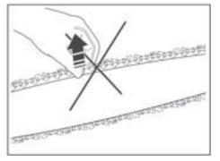
Using a screwdriver, make the chain run along the guides to check it moves smoothly without resistance.
