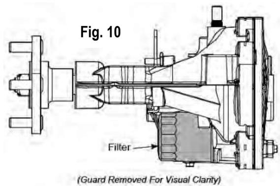
16. Push the neutral bypass levers back into place. Move the drive arms forward and backward 5 to 6 times slowly. Check the oil level and add oil as required after stopping the engine.
