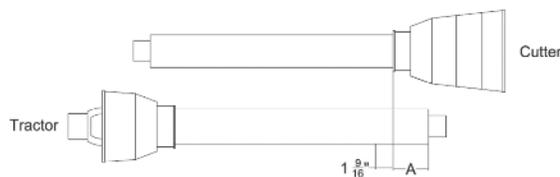
Do not use tractor if proper driveline engagement cannot be obtained through these methods. Connect driveline to tractor PTO shaft, making sure the spring-activated locking pin slides freely and locks driveline to PTO shaft.
