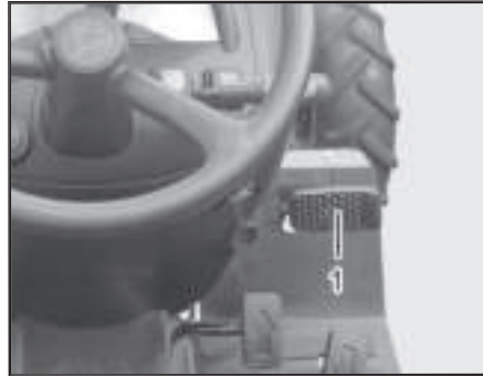
(1) Brake Pedal Free Play : 1.2 in~ 1.5 in (30~40 mm)
