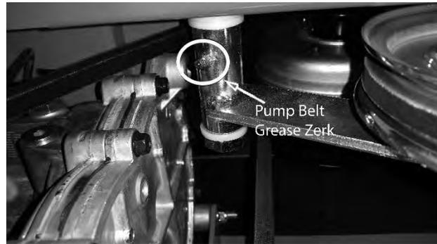
The deck belt tensioner is located at the rear of the deck and has a grease fitting on its pivot point. Grease at every engine oil change.
