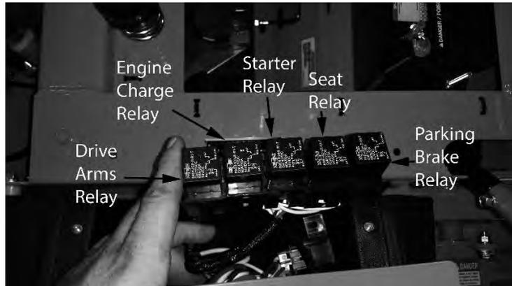
If you are having issues starting your mower ensure the signal wire is connected to your starter solenoid.
