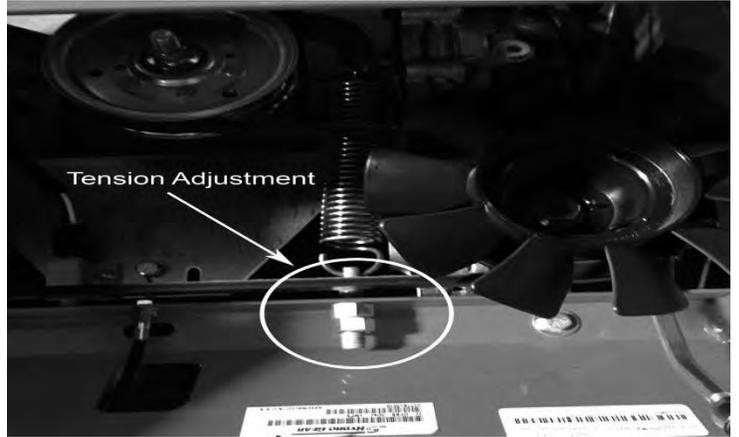
The tension should be adjusted so that there is between 50 to 55 lbs. of tension on the belt. This can be checked with a belt tension gauge as shown to the right.
