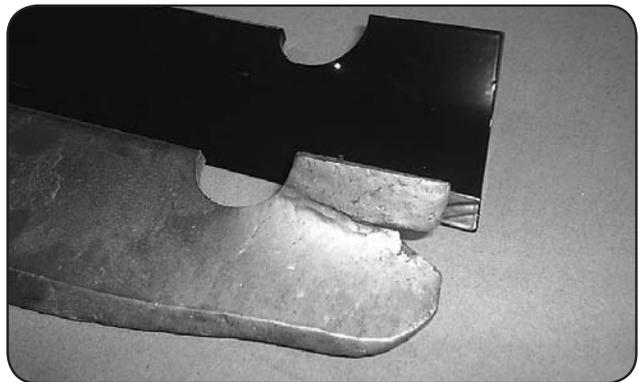
To change blades, it may be easier to use a piece of wood to keep the blade from turning so that the bolt can be loosened. Re-torque the blade bolts to 90-110 .lbs.
