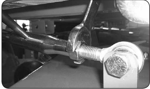
The deck spring tension is critical. If the tension is too much, it will cause the spring to break. If too loose, the belt can jump off or slip on the pulleys and cause a cut quality issue. With the deck up, the spring coil gap should be about .025" - .030" (about the thickness of a credit card). Spring tension adjustments can be made by sliding the bolt shown above forward or backward in the slot of the deck.
