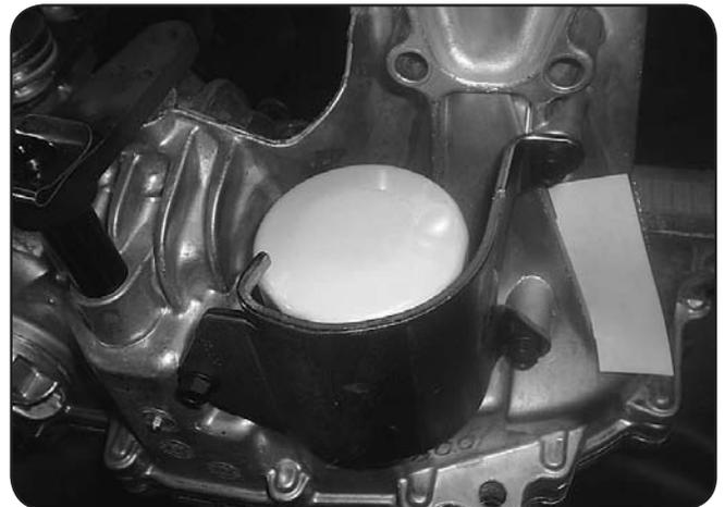
Shown right is the 5400 Outlaw transaxle. The large cap on the lower left is the filter housing cap.
