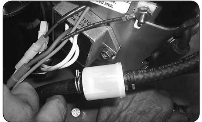
Remove and inspect air cleaner weekly. (More often in dusty conditions). Do not blow filter out with air pressure, this will cause the filter to be filled with tiny holes that will allow dirt to enter. Instead, tap filter on side to remove any debris. Replace at least once a year, more often in dusty conditions
