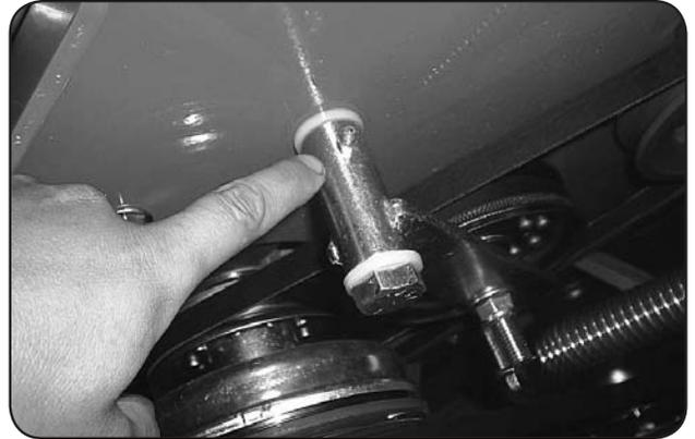
The deck belt tensioner is located at the rear of the deck and has a grease fitting on its pivot point. Grease at every engine oil change.
