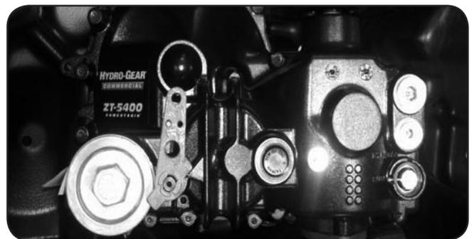
5400 filter housing cap. (do not over tighten)
