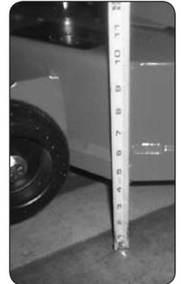
To check the level of the deck, start on a flat surface and set the air pressure in all four tires. Raise the deck up, and measure all four corners of the deck to see if it is level from left to right and front to back. All decks should be level from left to right and have a 1/8" pitch down in the front.
