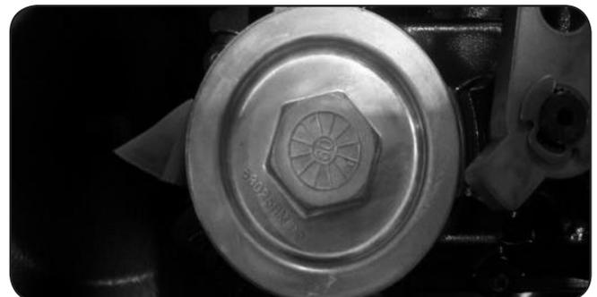
The check plug is located at the top center of the inside case of each transaxle (outlaw transaxles have this plug on the top). The transaxle can be filled with oil by removing these check plugs from both transaxles and pouring the oil in the hydro overflow tank, located behind the seat. Oil will begin to run out of the check plug holes when the transaxles are full. Use only 20w50 motor oil in the hydro system.
