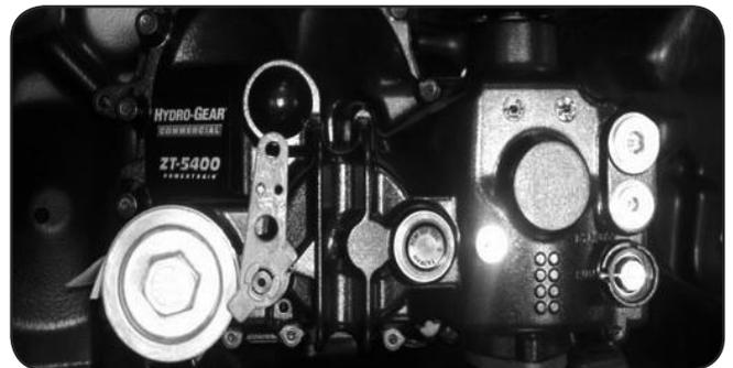
Filter housing cap. (do not over tighten)
