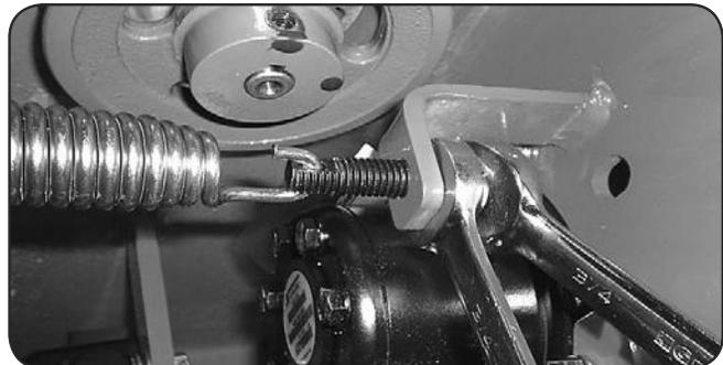
Tightening the two 3/4" jam nuts on the right side will increase the belt tension on all models. Factory setting is about .030" (about the thickness of a credit card) between coils as shown.
